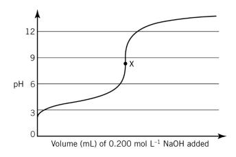
The graph shows the changes in pH that occur when 20.00 mL of 0.100 mol L<sup>-1</sup> benzoic acid solution in a conical flask is titrated with 0.200 mol L<sup>-1</sup> NaOH solution from a burette.
